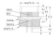
Part No.: MD08P3LPAB Contacts Poles: 08 Pin Connector Gender: Male connector Current Rating: 8 A Keyway Coding: A-Coding EMC Shielding: Half or partial shielded
