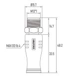
Part No.: MC05T1LSASS Contacts Poles: 05 Pin Connector Gender: Male connector Current Rating: 4 A Keyway Coding: A-Coding EMC Shielding: 360° fully shielded
