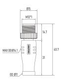
Part No.: MC05T1LSAP Contacts Poles: 05 Pin Connector Gender: Male connector Current Rating: 4 A Keyway Coding: A-Coding EMC Shielding: Un-shielded
