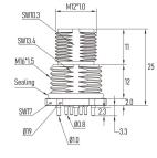
Part No.: MC08P1LPXSB16 Contacts Poles: 08 Pin Connector Gender: Male connector Current Rating: 0.5 A Wire Gauge (size): 26AWG/ 0.14mm<sup>2</sup> Keyway Coding: X-Coding EMC Shielding: 360° fully shielded
