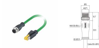
Part No.: RJ5EA1-MC04C1LSDSB22RGxxPFNI Contacts Poles: 04 Pin Cable Length: Customized lengthes Connector Gender: Male to male double ended Cable Jacket: PUR, halogen-free Voltage Rating: 250V EMC Shielding: 360° fully shielded Products Certification: UL Certified, CE/ EMC,
