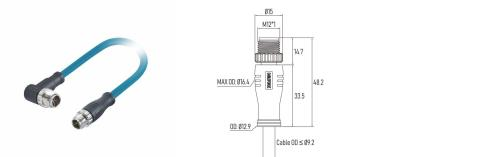
Part No.: MC08C5L/RSXSB26RLBxxPFN Contacts Poles: 08 Pin Cable Length: Customized lengthes Connector Gender: Male to male double ended Cable Jacket: PUR, halogen-free Voltage Rating: 48V EMC Shielding: 360° fully shielded Products Certification: CE/ EMC, IP67
