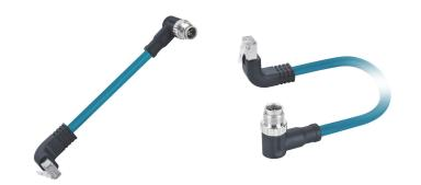
Part No.: RJ6AC1R-MC08C1LSXSB26RLBxx Contacts Poles: 08 Pin Cable Length: Customized lengthes Connector Gender: Male to male double ended Cable Jacket: PUR, halogen-free Voltage Rating: 48V EMC Shielding: 360° fully shielded Products Certification: UL Certified, CE/ EMC,
