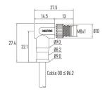
Part No.: MB04C5RSAB24CKxx Contacts Poles: 04 Pin Cable Length: Customized lengthes Connector Gender: Male to male double ended Cable Jacket: PVC Voltage Rating: 60V EMC Shielding: Un-shielded Products Certification: UL Certified, CUL Certif
