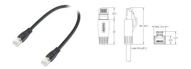
Part No.: RJ5EC5LI26CK03 Cable Length: 30 cm Connector Gender: Male to male double ended Wire Gauge (size): 26AWG/ 0.14mm<sup>2</sup> EMC Shielding: 360° fully shielded Straight/ 90° Angled: 180° Straight
