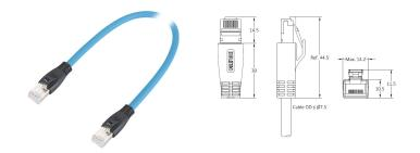
Part No.: RJ5EC5LI26CB03 Cable Length: 30 cm Connector Gender: Male to male double ended Wire Gauge (size): 26AWG/ 0.14mm<sup>2</sup> EMC Shielding: 360° fully shielded Straight/ 90° Angled: 180° Straight
