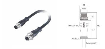
Part No.: MC04C1P2LSDSB22RKxx-F5 Cable Length: Customized lengthes Connector Gender: Male to female connector, c Wire Gauge (size): 26AWG/ 0.14mm<sup>2</sup> Keyway Coding: D-Coding EMC Shielding: 360° fully shielded Straight/ 90° Angled: 180° Straight Drag chain bending life: 5 million cycles
