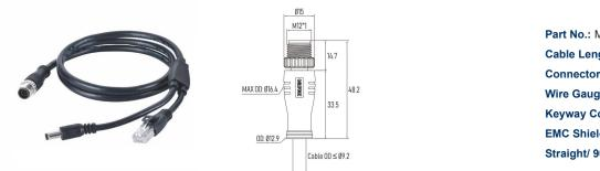
Part No.: MC08C1LSASB24CK15-DC/RJ45 Cable Length: 1.5 m Connector Gender: Male connector Wire Gauge (size): 24AWG/ 0.25mm<sup>2</sup> Keyway Coding: A-Coding EMC Shielding: 360° fully shielded Straight/ 90° Angled: 180° Straight
