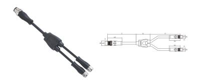
Part No.: MC04C1LSAB22CB01Y02MB04C2 Contacts Poles: 04 Pin Cable Length: 30 cm Connector Gender: Male connector, Female co Cable Jacket: PVC Voltage Rating: 60V EMC Shielding: Un-shielded Products Certification: CE/ EMC, IP67
