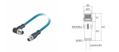
Part No.: MC08C5L/RSXSB26RLBxxPFN Cable Length: Customized lengthes Connector Gender: Male to male double ended Wire Gauge (size): 26AWG/ 0.14mm<sup>2</sup> Keyway Coding: X-Coding EMC Shielding: 360° fully shielded Straight/ 90° Angled: 180° Straight, 90° right an Drag chain bending life: 2 million cycles
