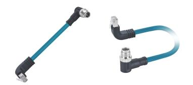
Part No.: RJ6AC1R-MC08C1LSXSB26RLBxx Cable Length: Customized lengthes Connector Gender: Male to male double ended Wire Gauge (size): 26AWG/ 0.14mm<sup>2</sup> Keyway Coding: X-Coding EMC Shielding: 360° fully shielded Straight/ 90° Angled: 90° right angled
