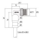
Part No.: MC04C1LSDSB24RG18-RJ5E Cable Length: Customized lengthes Connector Gender: Male to male double ended Wire Gauge (size): 24AWG/ 0.25mm<sup>2</sup> Keyway Coding: D-Coding EMC Shielding: 360° fully shielded Straight/ 90° Angled: 180° Straight
