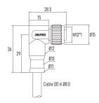
Part No.: MC04C2RCSB16RK10-CEE7 Contacts Poles: 03 Pin, 3 + PE Cable Length: 1 m Connector Gender: Female connector Cable Jacket: PUR, halogen-free Voltage Rating: 630V EMC Shielding: Un-shielded Products Certification: CE/ EMC, IP67, IP69K
