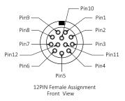
Part No.: LF10WBJ-12S-2M Contacts Poles: 12 Pin Cable Length: 2 m Connector Gender: Male connector Cable Jacket: PVC Voltage Rating: 30V EMC Shielding: 360° fully shielded
