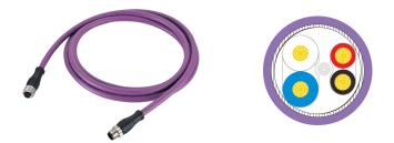
Part No.: MC05C3LSAB22CV100-CAN Contacts Poles: 05 Pin Cable Length: 10 m Connector Gender: Male to female connector, c Cable Jacket: PVC Voltage Rating: 60V EMC Shielding: Half or partial shielded Products Certification: UL Certified, CUL Certif
