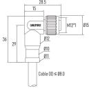
Part No.: MC05C4RSAB22RK20 Contacts Poles: 05 Pin Cable Length: 2 m Connector Gender: Female to female connecto Cable Jacket: PUR, halogen-free Voltage Rating: 60V EMC Shielding: Un-shielded Products Certification: UL Certified, CUL Certif
