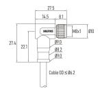
Part No.: MB05C4RSBB24RK30 Contacts Poles: 05 Pin Cable Length: 3 m Connector Gender: Female to female connecto Cable Jacket: PUR, halogen-free Voltage Rating: 30V EMC Shielding: Un-shielded Products Certification: CE/ EMC, IP67, IP69K
