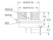
Part No.: MD06P2LPAB Contacts Poles: 06 Pin Connector Gender: Female connector Current Rating: 8 A Keyway Coding: A-Coding EMC Shielding: Half or partial shielded
