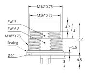
Part No.: MD07P1LPBB Contacts Poles: 07 Pin Connector Gender: Male connector Current Rating: 8 A Keyway Coding: B-Coding EMC Shielding: Half or partial shielded
