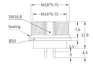
Part No.: MD12P2LPAB Contacts Poles: 12 Pin Connector Gender: Female connector Current Rating: 4 A Keyway Coding: A-Coding EMC Shielding: Half or partial shielded
