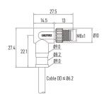
Part No.: MB04C1RSAB-24xx xx Contacts Poles: 04 Pin Connector Gender: Male connector Cable Jacket: PVC, PUR, halogen-free, Custom Current Rating: 3 A Wire Gauge (size): 24AWG/ 0.25mm<sup>2</sup> Keyway Coding: A-Coding EMC Shielding: Un-shielded
