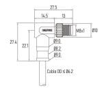
Part No.: MB03C1RSASB-24xx xx Contacts Poles: 03 Pin Connector Gender: Male connector Cable Jacket: PVC, PUR, halogen-free, Custor Current Rating: 3 A Wire Gauge (size): 24AWG/ 0.25mm<sup>2</sup> Keyway Coding: A-Coding EMC Shielding: 360° fully shielded
