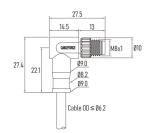
Part No.: MB05C1RSBB-24xx xx Contacts Poles: 05 Pin Connector Gender: Male connector Cable Jacket: PVC, PUR, halogen-free, Custom Current Rating: 3 A Wire Gauge (size): 24AWG/ 0.25mm<sup>2</sup> Keyway Coding: B-Coding EMC Shielding: Un-shielded
