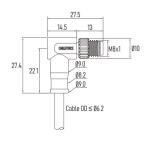
Part No.: MB04C1RSASB-24xx xx Contacts Poles: 04 Pin Connector Gender: Male connector Cable Jacket: PVC, PUR, halogen-free, Custorr Current Rating: 3 A Wire Gauge (size): 24AWG/ 0.25mm<sup>2</sup> Keyway Coding: A-Coding EMC Shielding: 360° fully shielded
