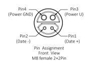
Part No.: MBH22C2LSASB-22xx xx Contacts Poles: 04 Pin, 2 + 2 + PE Connector Gender: Male connector
