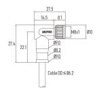
Part No.: MB03C2RSAB-24xx xx Contacts Poles: 03 Pin Connector Gender: Female connector Cable Jacket: PVC, PUR, halogen-free, Custom Current Rating: 3 A Wire Gauge (size): 24AWG/ 0.25mm<sup>2</sup> Keyway Coding: A-Coding EMC Shielding: Un-shielded
