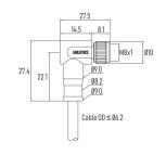
Part No.: MB06C2RSAP-26xx xx Contacts Poles: 06 Pin Connector Gender: Female connector Cable Jacket: PVC, PUR, halogen-free, Custorr Current Rating: 1.5 A Wire Gauge (size): 26AWG/ 0.14mm<sup>2</sup> Keyway Coding: A-Coding EMC Shielding: Un-shielded
