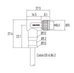
Part No.: MB08C2RSASB-26xx xx Contacts Poles: 08 Pin Connector Gender: Female connector Cable Jacket: PVC, PUR, halogen-free, Custorr Current Rating: 1.5 A Wire Gauge (size): 26AWG/ 0.14mm<sup>2</sup> Keyway Coding: A-Coding EMC Shielding: 360° fully shielded
