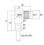
Part No.: MC04C2RSASB-22xx xx Contacts Poles: 04 Pin Connector Gender: Female connector Cable Jacket: PVC, PUR, halogen-free, TPE 90 Current Rating: 4 A Wire Gauge (size): 22AWG/ 0.34mm<sup>2</sup> Keyway Coding: A-Coding EMC Shielding: 360° fully shielded
