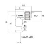
Part No.: MC03C2RSASB-22xx xx Contacts Poles: 03 Pin Connector Gender: Female connector Cable Jacket: PVC, PUR, halogen-free, TPE 90 Current Rating: 4 A Wire Gauge (size): 22AWG/ 0.34mm<sup>2</sup> Keyway Coding: A-Coding EMC Shielding: 360° fully shielded
