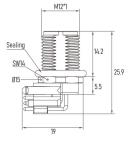
Part No.: MC04P1RPAB12 Contacts Poles: 04 Pin Connector Gender: Male connector Current Rating: 4 A Keyway Coding: A-Coding EMC Shielding: Un-shielded
