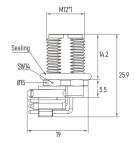
Part No.: MC08P1RPAB12 Contacts Poles: 08 Pin Connector Gender: Male connector Current Rating: 2 A Keyway Coding: A-Coding EMC Shielding: Un-shielded
