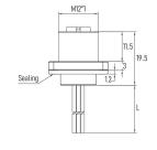
Part No.: MC05P2LPABF-22W30 Contacts Poles: 05 Pin Connector Gender: Female connector Current Rating: 4 A Wire Gauge (size): 22AWG/ 0.34mm<sup>2</sup> Keyway Coding: A-Coding EMC Shielding: Un-shielded
