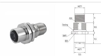
Part No.: MC04P7ABP9 Contacts Poles: 04 Pin Connector Gender: Male connector, Female co Current Rating: 4 A Keyway Coding: A-Coding EMC Shielding: 360° fully shielded
