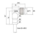
Part No.: MC05C2RSBB-22xx xx-PFB Contacts Poles: 05 Pin Connector Gender: Female connector Cable Jacket: PVC, PUR, halogen-free, Custom Current Rating: 4 A Wire Gauge (size): 22AWG/ 0.34mm<sup>2</sup> Keyway Coding: B-Coding EMC Shielding: 360° fully shielded
