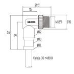
Part No.: MC04C1RSDSB-22xx xx-PFN Contacts Poles: 04 Pin Connector Gender: Male connector Cable Jacket: PVC, PUR, halogen-free, Custor Current Rating: 4 A Wire Gauge (size): 22AWG/ 0.34mm<sup>2</sup> Keyway Coding: D-Coding EMC Shielding: 360° fully shielded
