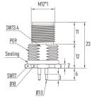
Part No.: MC04P1LPDBxx Contacts Poles: 04 Pin Connector Gender: Male connector Current Rating: 4 A Keyway Coding: D-Coding EMC Shielding: Un-shielded
