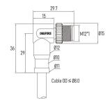
Part No.: MC04C1RCSB-16xx xx Contacts Poles: 3 + PE Connector Gender: Male connector Cable Jacket: PVC, PUR, halogen-free, Custorr Current Rating: 12 A Wire Gauge (size): 16AWG/ 1.5mm<sup>2</sup> Keyway Coding: S-Coding EMC Shielding: Un-shielded
