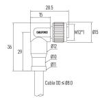
Part No.: MC04C2RCSB-16xx xx Contacts Poles: 3 + PE Connector Gender: Female connector Cable Jacket: PVC, PUR, halogen-free, Custorr Current Rating: 12 A Wire Gauge (size): 16AWG/ 1.5mm<sup>2</sup> Keyway Coding: S-Coding EMC Shielding: Un-shielded
