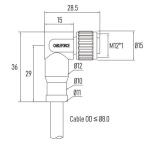
Part No.: MC04C2RCTSB-16xx xx Contacts Poles: 04 Pin Connector Gender: Female connector Cable Jacket: PVC, PUR, halogen-free, Custor Current Rating: 12 A Wire Gauge (size): 16AWG/ 1.5mm<sup>2</sup> Keyway Coding: T-Coding EMC Shielding: 360° fully shielded
