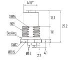
Part No.: MC05P2LPKBxx Contacts Poles: 05 Pin, 4 + PE Connector Gender: Female connector Current Rating: 16 A Keyway Coding: K-Coding EMC Shielding: Un-shielded
