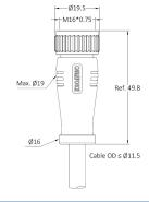
Part No.: MD12C2LSASB-22xx xx Contacts Poles: 12 Pin Connector Gender: Female connector Cable Jacket: PVC, PUR, halogen-free, Custor Current Rating: 4 A Wire Gauge (size): 22AWG/ 0.34mm<sup>2</sup> Keyway Coding: A-Coding EMC Shielding: 360° fully shielded
