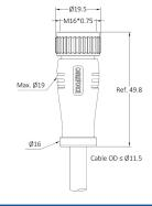
Part No.: MD08C2LSASB-18xx xx Contacts Poles: 08 Pin Connector Gender: Female connector Cable Jacket: PVC, PUR, halogen-free, Custor Current Rating: 8 A Wire Gauge (size): 18AWG/ 0.75mm<sup>2</sup> Keyway Coding: A-Coding EMC Shielding: 360° fully shielded
