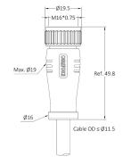
Part No.: MD06C2LSASB-18xx xx Contacts Poles: 06 Pin Connector Gender: Female connector Cable Jacket: PVC, PUR, halogen-free, Custor Current Rating: 8 A Wire Gauge (size): 18AWG/ 0.75mm<sup>2</sup> Keyway Coding: A-Coding EMC Shielding: 360° fully shielded
