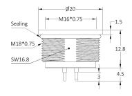
Part No.: MD05P4LPAB Contacts Poles: 05 Pin Connector Gender: Female connector Current Rating: 8 A Keyway Coding: A-Coding EMC Shielding: Half or partial shielded
