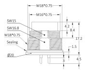
Part No.: MD08P1LPAB Contacts Poles: 08 Pin Connector Gender: Male connector Current Rating: 8 A Keyway Coding: A-Coding EMC Shielding: Half or partial shielded
